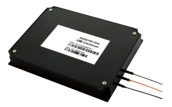
UMI optical interleaver is a 3-port passive fiber-optic device that is used to separate Dense Wavelength-Division Multiplexing (DWDM) channels into two groups of signal streams (odd and even channels) in an interleaving way. UMI optical interleaver uses an innovative design that features wide stopband and higher channel isolation. It provides the best solution to expand wavelength channel counts in DWDM system.
